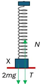
The tension force  $T$  is downward. The spring is compressed so the tension is upwards at the top end and downwards at the lower end. Hence,
